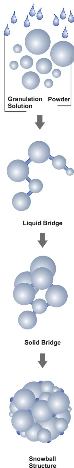
Fig. 3: Wet Granulation Process
